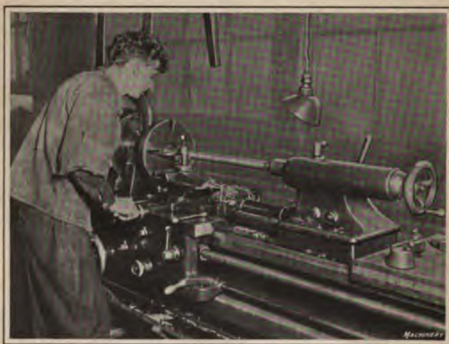
Fig. 3. Compound Rest set Parallel to Axis of Screw for Adjusting Tool when Cutting Multiple Thread
